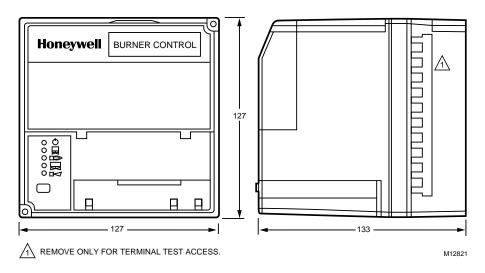
Fig. 1 Mounting dimensions of relay module and wiring subbase in millimeters only.
